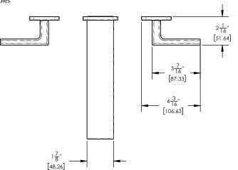
Spout Reach: 8" Installation Type: Wall Mounted Primary Material: Brass Valve Material: Ceramic Flow Restriction: Full Flow Water Pressure Maximum: 85 PSI Water Pressure Minimum: 20 PSI Water Pressure Recommended: 60 PSI
